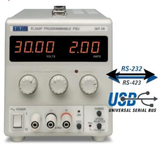
The EL302P is a digitally controlled version of the EL302 with an isolated RS-232 interface. It offers a low-cost solution for a basic programmable PSU and will be sufficient for many applications where the sophistication and complexity of GPIB is not needed.
